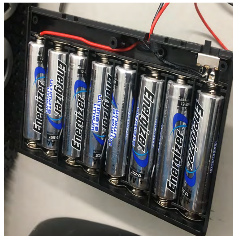
Power source, two 8AA battery packs
